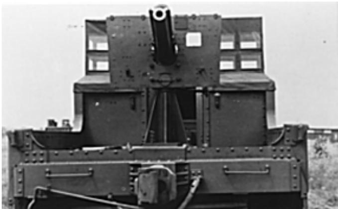
A 75 mm gun mounted on a gondola car. There was one such gun at each end of the train.
