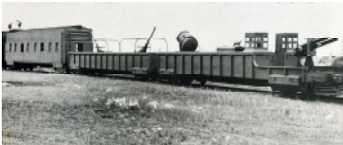
Viewed from the steam-style pilot at its front end, Canada's Armoured Train bristled with 75mm pivot-mounted gun, aircraft searchlight, a pair of 45mm anti-aircraft guns, and light machinegun mounts on the converted GTW auto carriers.
